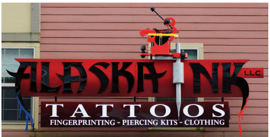
The main sign is 3-by-16-ft., with 35-by-41-in. tattoo gun. "We used a 3mm gloss black Dibond aluminum composite material [ www.graphicdisplayusa.com ] and ¼-in. white acrylic for the lettering," says Jeremy Barry, Sign Pro of Ketchikan, Ketchikan, Alaska. "The fade on the background was done with 1 Shot Bright Red enamel [ www.1shot.com ]. We used 15 lb. Sign Foam HDU [ www.signfoam.com ] for the body and grip of the tattoo gun, and PVC pipe for the machine handle. The gun is finished with 1 Shot enamel, too."
