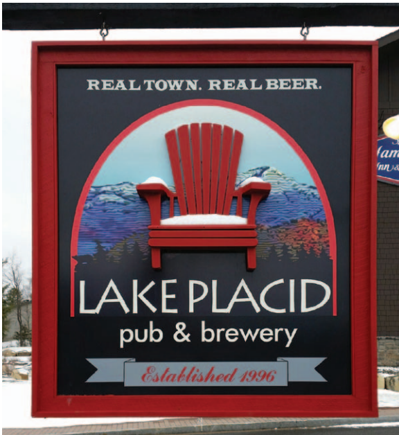
The background graphic is a digital print on 3M 180c film with 3M 8518 laminate on 3/4-in. PVC panel. The chair is hand carved HDU board, and the frame is cedar. "Yes, that is real snow piled on the chair!" says Laura Walker, Laura's Custom Artworks, Lake Placid, New York.
