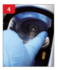
Track filling disc edge and press down firmly, ensuring disc is firmly in place.
