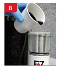
Fill plastic filling cup to filling line with mixed color.
