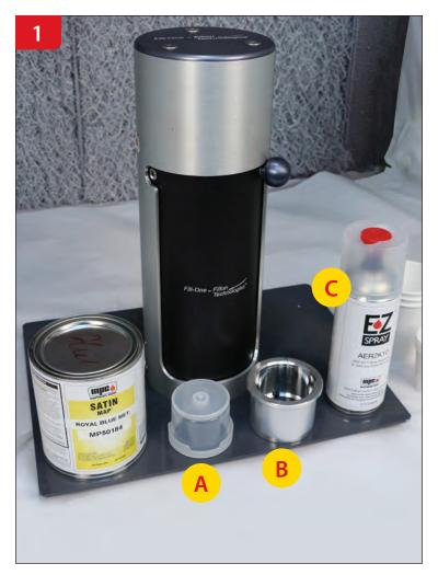
Check that you have the following equipment: Plastic Filling Cup, Adapter Ring, Filling Disc (A), Metal Cylinder Cup (B), Cap with Red Plunger (C)
