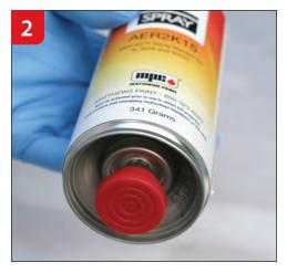
Attach red plunger to drive pin on bottom of can.
