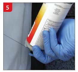
Remove top plastic filling cup with color indicator. Facing can away from you, turn can upside down and purge can until a smooth spray pattern is achieved.
