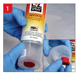
Remove bottom cap with red plunger. Remove red plunger from bottom cap.
