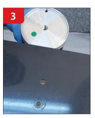
Align the center hole and offset hole in the base plate with the center hole and offset hole in the filling machine.
