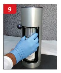
Insert aerosol can with filled metal cylinder cup into machine.
