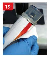
Pull black and white label off of aerosol can, revealing the color label.
