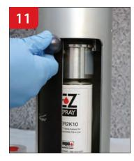
Close machine's door to initiate filling (about 3-6 seconds).
