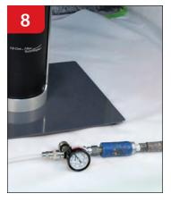
Make all air line connections from machine to gauge and air supply as shown above.
