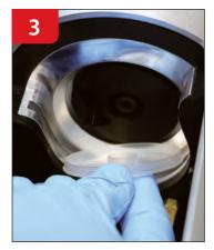
Place filling disc on press-in stamp on inside of filling machine.
